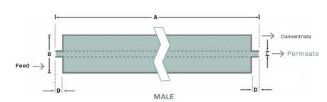
a) This model has a fiberglass outerwrap and diamond shaped feed spacers.
